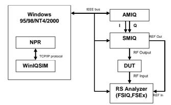
Fig. 1 Connecting Instruments
