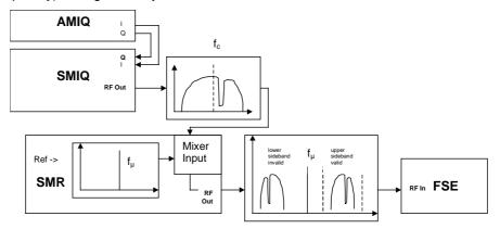
Fig. 26 NPR with Microwaves
